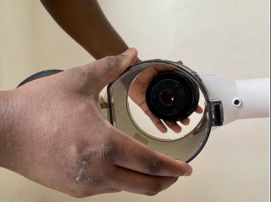
Remove the black part by gently pushing from inside of the canister.
