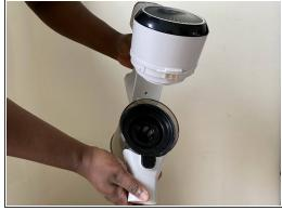
After emptying the debris, hold down the black button, then twist and pull the canister out.
