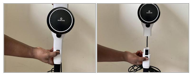
Hold down the black button to remove the white motor unit above and gently pull the motor unit upwards.
