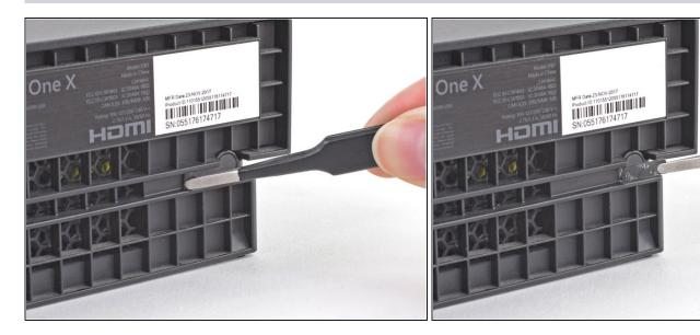
Use blunt <u>tweezers</u> to peel off the sticker covering the right-side screw on the back of the console.
