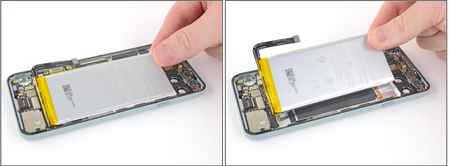
**⚠ Do not reuse the battery if it has been deformed or damaged, as doing so is a potential safety hazard. Replace it with a new battery.**
