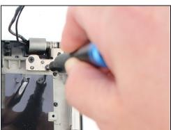
• Using the Phillips #1 screwdriver, remove two 4.3 mm screws from each hinge (four total).
