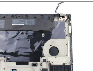
• Remove the cables from the cable guides.
