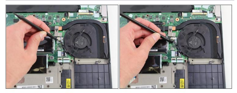
• Use the black nylon spudger to slide the fan connector parallel to the motherboard and out of its socket on the motherboard.
