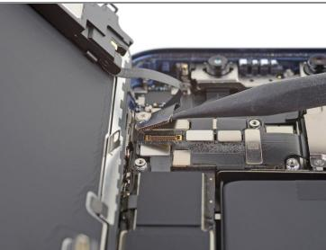
• Use a spudger or a fingernail to disconnect the front sensor assembly cable connector.
