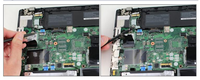
• Insert the point of a spudger under one of the antenna cables close to the connector. Pry straight up to disconnect the cable off of the Wi-Fi card.
