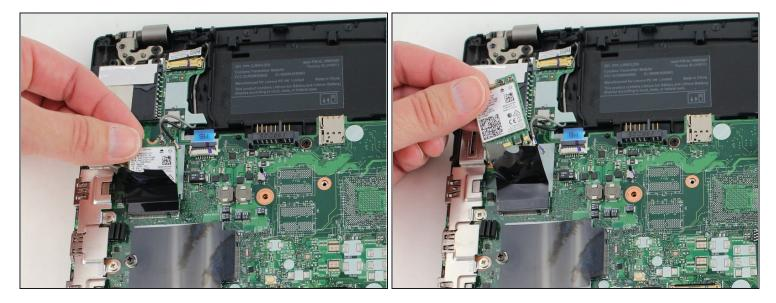
• Slide the Wi-Fi card out from the slot to remove it from the board.
