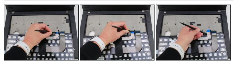
• Using the black nylon spudger, unlock the second ribbon connector and slide it out from the port.
