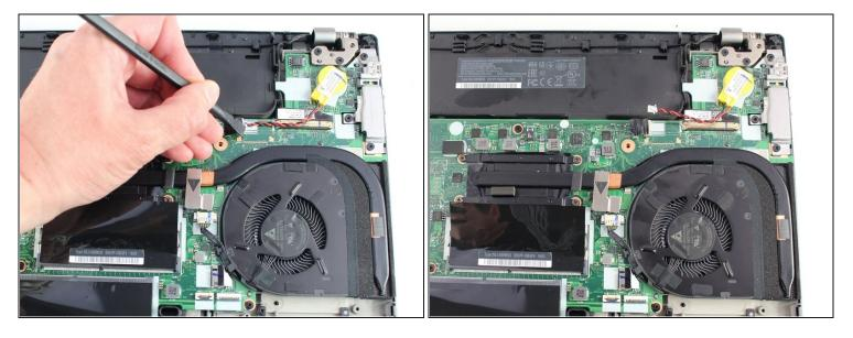
• Using an IC extractor or black nylon spudger, unplug the connector from the socket on the motherboard.
