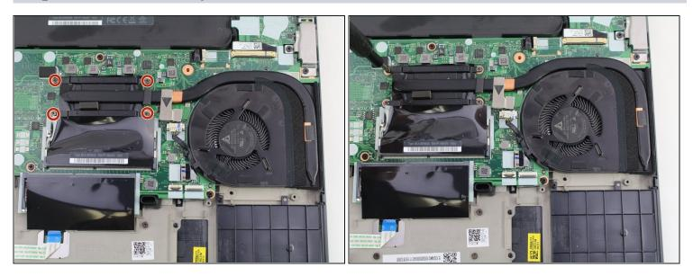
• Using the Phillips #1 screwdriver, loosen the four captive screws in the arm of the heatsink.
