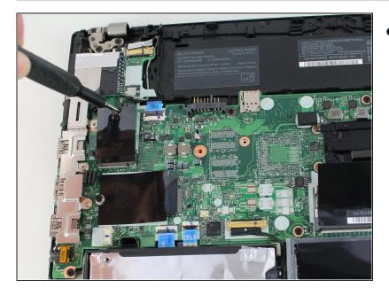
Using the Phillips #1 screwdriver, remove the single 3.6 mm screw at the top of the Wi-Fi card attaching it to the motherboard.
