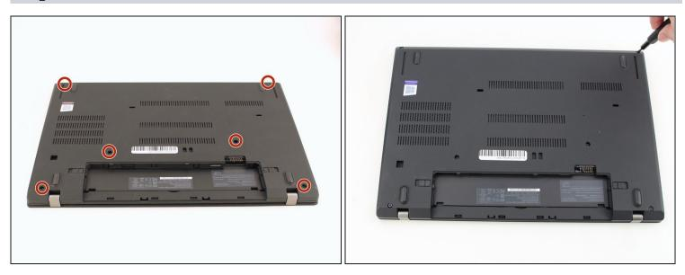
• Using the Phillips #1 screwdriver, loosen the six captive screws.
