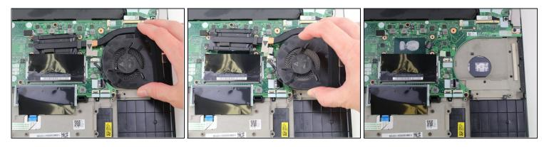
• Lift the fan assembly off of the board.
