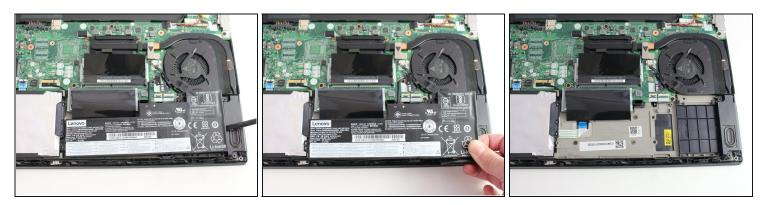
• Using the black nylon spudger, wedge the battery up from the case and lift it out.
