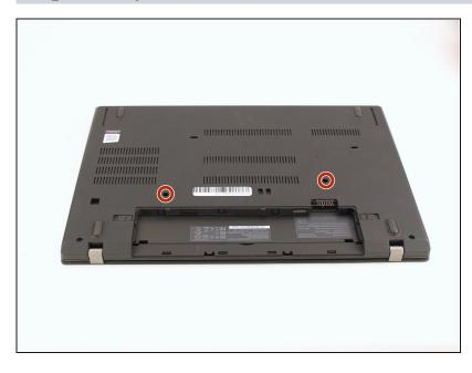
• Use the Phillips #1 screwdriver to loosen the two screws parallel to the battery compartment.
