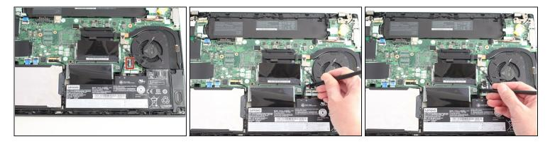
• Use the spudger to slide the battery socket connector parallel to the motherboard and out of its socket on the motherboard.
