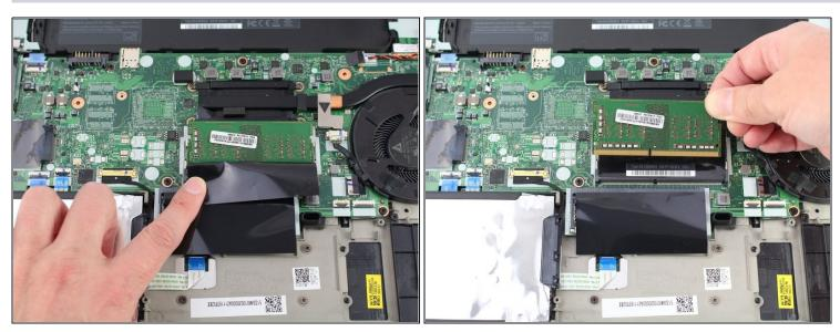
• Slide the RAM stick out from the memory module slot.
