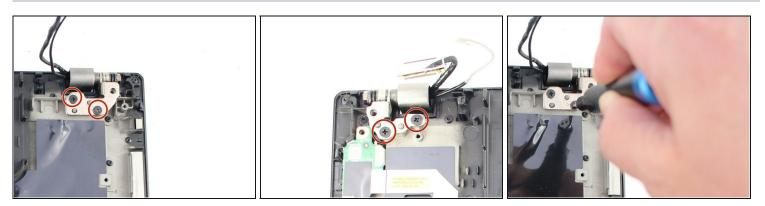
• Using the Phillips #1 screwdriver, remove two 4.3 mm screws from each hinge (four total).
