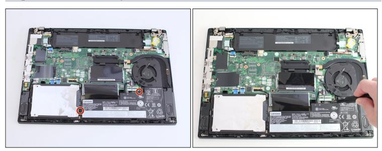
• Using the Phillips #1 screwdriver, remove the two 4.6 mm screws securing the internal battery to the frame.
