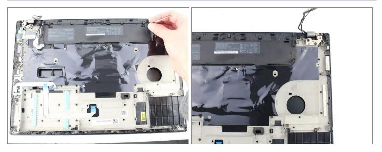
• Remove the cables from the cable guides.
