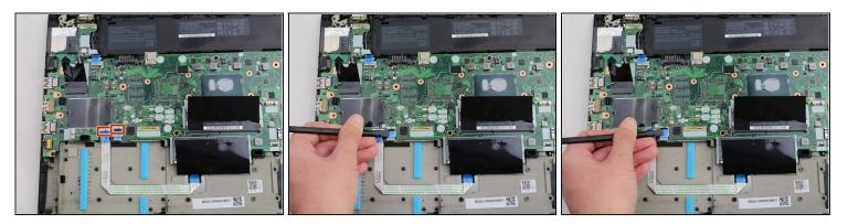
• Using the black nylon spudger, remove the NFC cable connector and trackpad connector from the motherboard.
