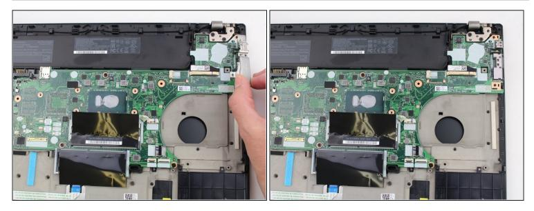
• Lift the I/O bracket off the motherboard.
