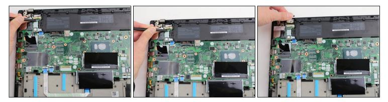
• Using the black nylon spudger, disconnect the LCD cable from the motherboard.
