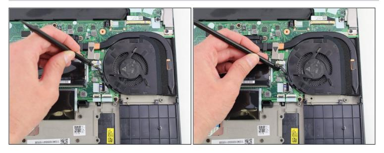
• Use the black nylon spudger to slide the fan connector parallel to the motherboard and out of its socket on the motherboard.
