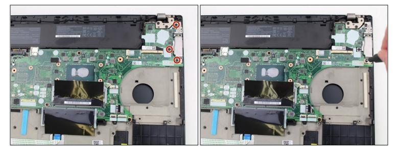
• Using the Phillips #1 screwdriver, remove three 4.6 mm screws from the I/O bracket.
