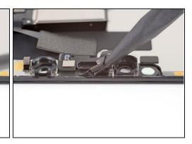
• Use the point of a spudger to lift and separate the ambient light sensor from its notch in the front panel.
