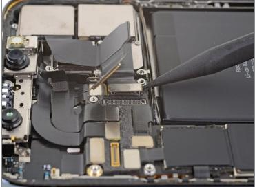
• Use a spudger or a fingernail to disconnect the second camera cable connector by prying it straight up from its socket.
