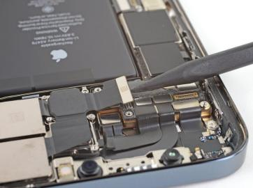
• Use a spudger or a fingernail to disconnect the first camera cable connector by prying it straight up from its socket.
