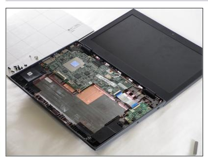
• The battery is now loose and can be removed from the laptop.
