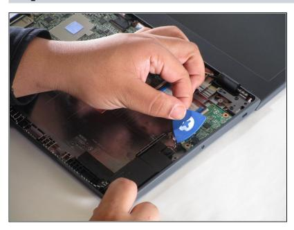
Using a plastic opening pick, remove the connection between the aux port and the speakers.
