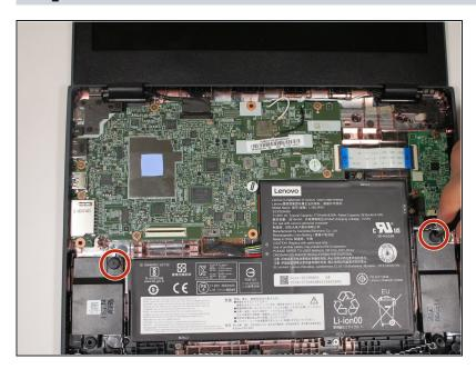
Remove the two 2 mm Phillips #0 screws holding both of the speakers in.
