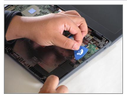
Using an opening pick, disconnect the speakers from the headphone jack.
