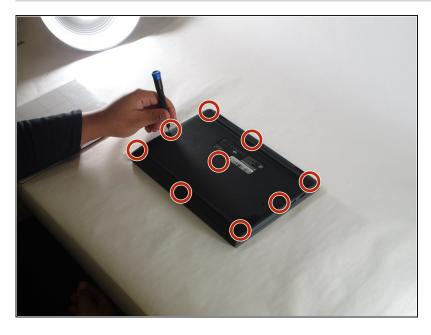
Remove the nine 6 mm screws from the back of the laptop using a Phillips #0 screwdriver.
