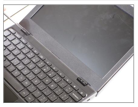
• Insert the spudger into the gap between the hinges and pull up to detach the connections.
