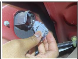
• Pull on the gray plastic part of the tail light assembly to remove it from the car.
