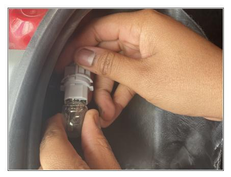
Unscrew the bulb from its socket and replace it with a new one.
