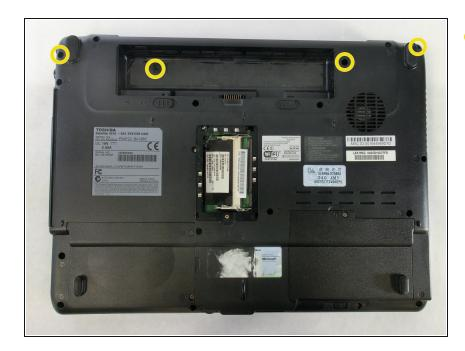
Unscrew the 4 highlighted screws with a PH1 screwdriver.
