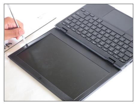
Using a spudger, go along the edge of the screen and pop the connections between the cover and the back side out.
