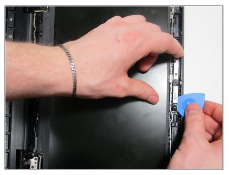
Using the opening pick, pry the camera from the front of the laptop.
