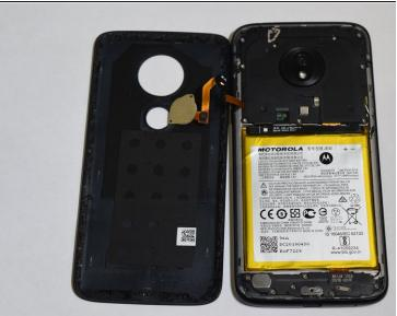
• Use the iFixit pick and the iFixit opening tool to pull the fingerprint scanner off of the back case.
