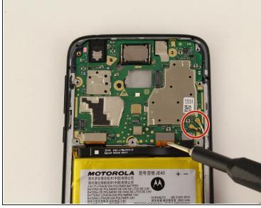
• Once the motherboard cover is removed, disconnect the four ribbon cables and the two wires attached to the motherboard.
