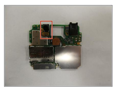
Separate the front facing camera from the motherboard while removing the adhesive. To reassemble your device, follow these instructions in reverse order.
