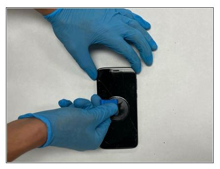
Use the suction cup tool to lift the screen without damaging or scratching screen.
