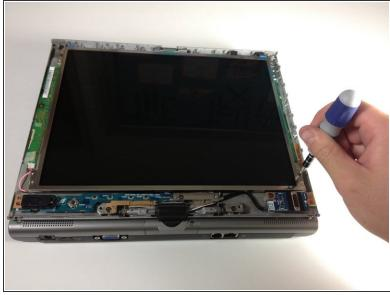
Remove the four 5 mm screws with a Phillips #1 screwdriver, each located at the four corners of the screen.
