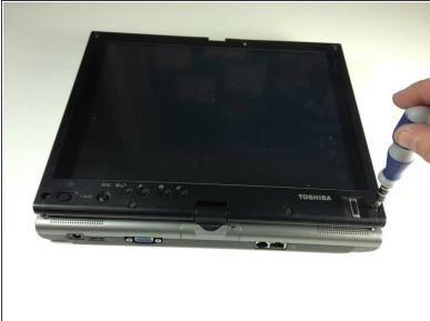
Remove all six 3.8mm screws from the screen using a #1 Phillips screwdriver.
