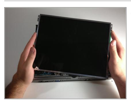
At this point, the screen should be completely disconnected from the rest of the laptop.
