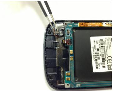
• On the right from the lever, use the tweezers to unclip the black connector.
