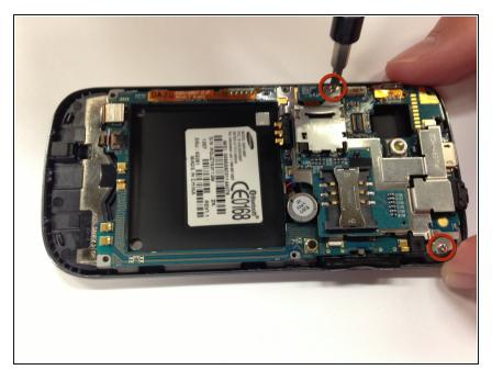
Using a Phillips #00 screwdriver, remove the two 3.8mm screws.
