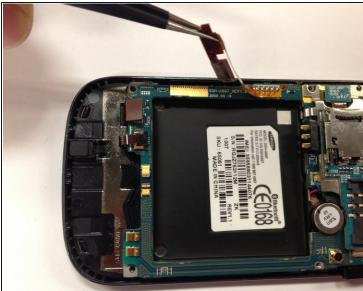
• Use the tweezers to unclip the orange ribbon cable from the left side of the phone.
