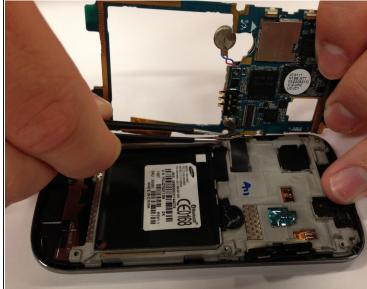
⚠ DO NOT remove the motherboard completely. One more clip on the motherboard's backside needs to be removed.
