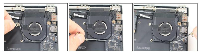
Unwind the black and white coaxial cables from the hooks on the right fan casing.
