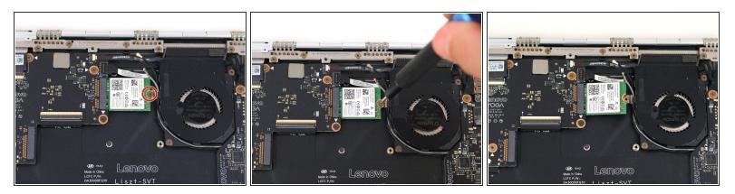
• Using a Phillips #00 screwdriver, remove the 2.2 mm screw holding down the Wi-Fi card.
