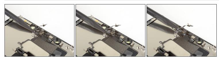
• Use the point of a spudger to lift and separate the microphone from its notch in the front panel.
