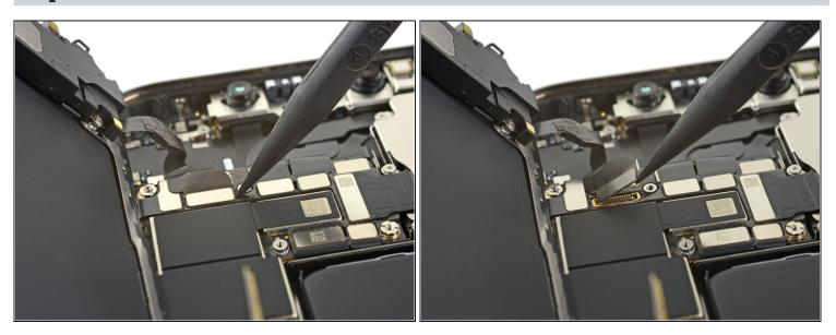
Use a spudger or a fingernail to disconnect the front sensor assembly cable connector.
