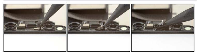
• Use the point of a spudger to lift and separate the ambient light sensor from its notch in the front panel.
