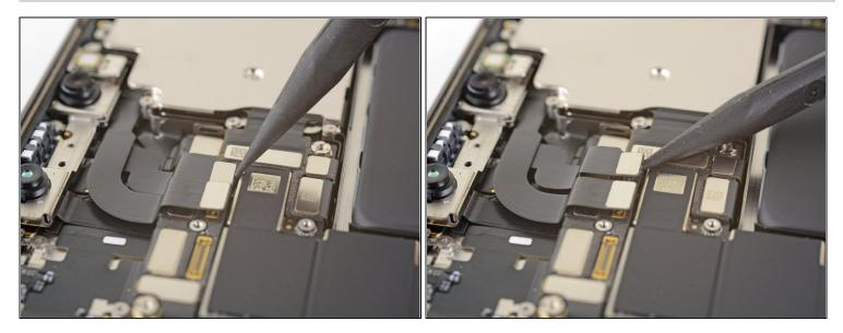
• Use a spudger or a fingernail to disconnect the Face ID dot projector cable from its socket on the logic board.
