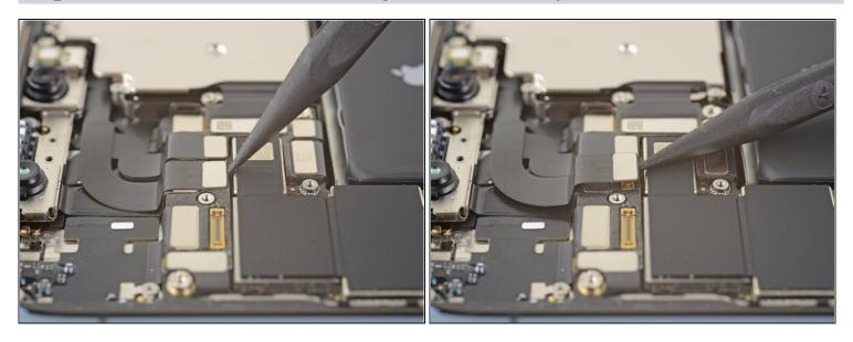
• Use a spudger or a fingernail to disconnect the Face ID sensor cable from its socket on the logic board.
