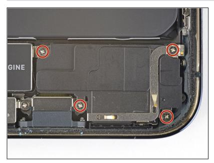
Use a Phillips driver to remove the four 1.4 mm screws securing the loudspeaker.
