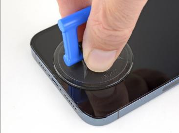
• If you're using a single suction handle, apply it to the bottom edge of the phone, while avoiding the very edge of the glass.
