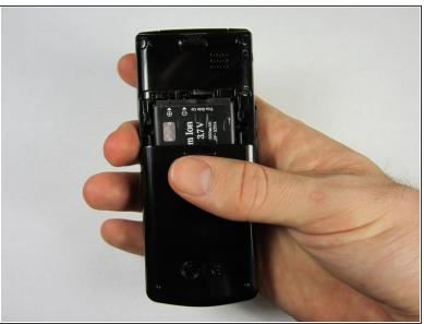
Use your thumb to press down and slide off the back cover of the phone.
