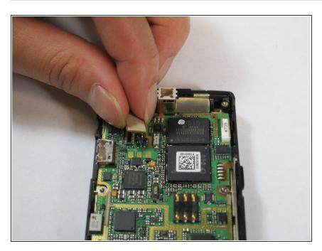
Remove the plastic tab connecting the screen to the motherboard by pulling the tab up from the board.
