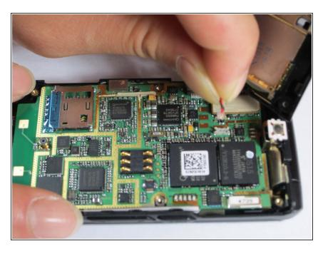
Gently pull the wire up from the motherboard, separating the back of the phone and the motherboard.
