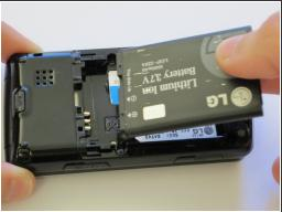
• Take out the battery by levering it out towards the bottom of the phone.
