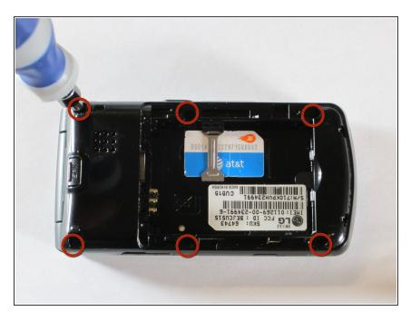
Remove six 3.0 mm Phillips #00 screws from the back of the phone.
