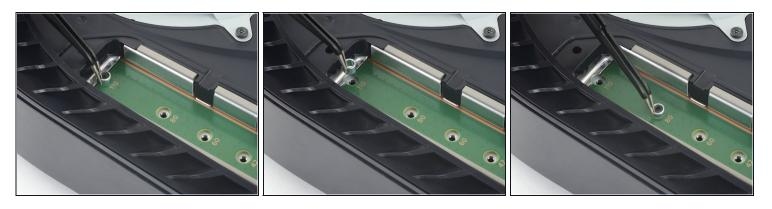
Use a pair of tweezers to lift and move the spacer to the appropriate slot for your chosen M.2 SSD.
