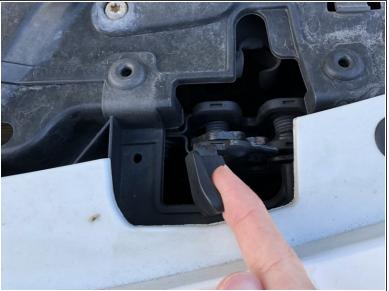
Open the hood by pushing left on the hood latch.
