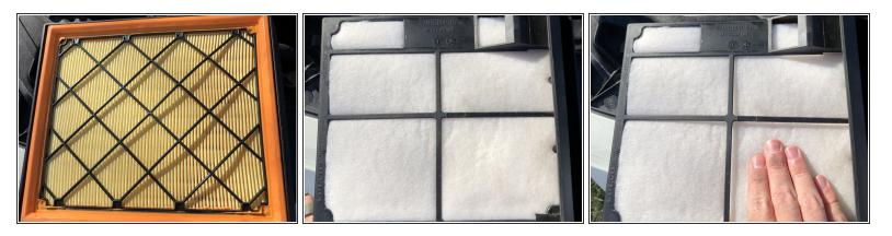
Take out the old air filter by flipping it over and pushing it out through the bottom.
