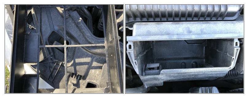
• Clean out any extra debris that maybe in the air filter holder or inside the engine.
