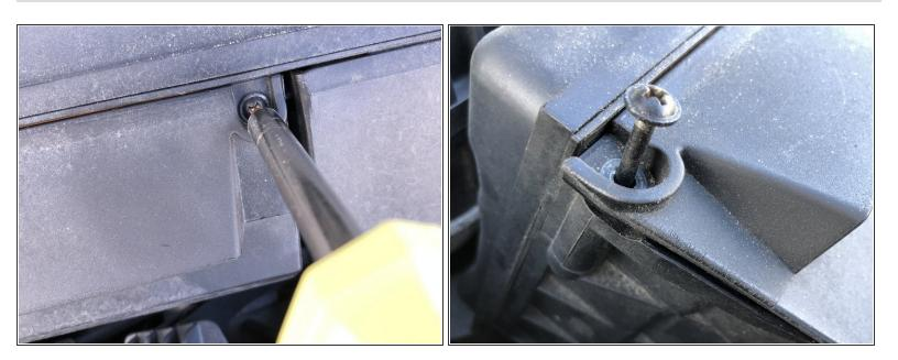
Remove the two 2 inch screws from the case using the Phillips #2 screwdriver.
