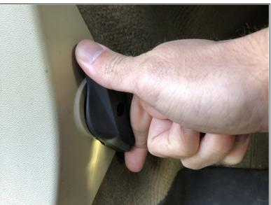
Unlatch the hood by pulling on the hood release lever.
