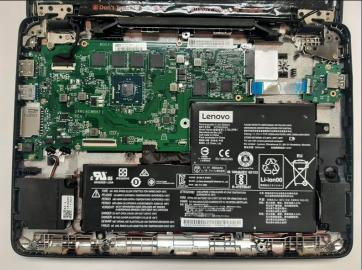
• Disconnect the two black connectors on the bottom left side of the motherboard by pulling back on the lip with a plastic opening tool.
