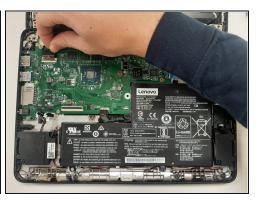
Disconnect the video cable by lifting upwards on the black tab using a plastic opening tool and pulling the cable out.
