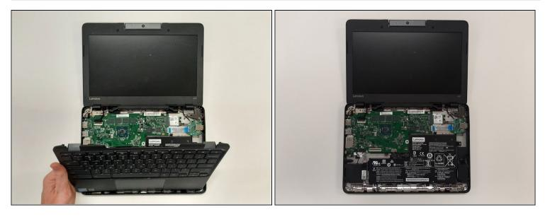
Lift the keyboard panel from the case and fully remove it from the device.
