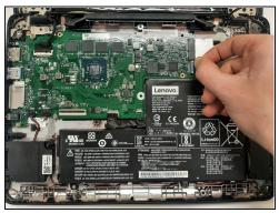
• Remove the USB ribbon cable by lifting up on the white tab using a plastic opening tool and then pulling the cable out.
