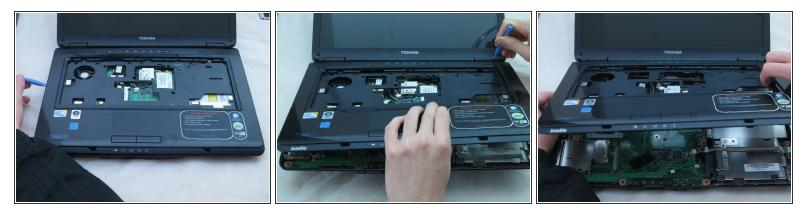
Separate the laptop upper casing from the lower casing by using an opening tool around the sides of the case to pry it apart.
