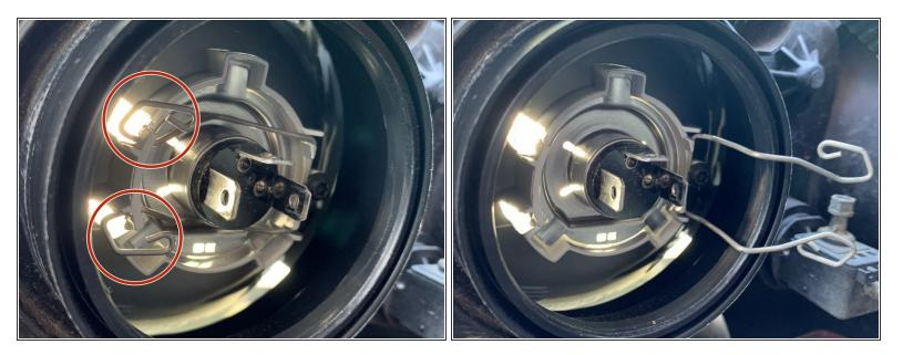
• Unlatch the bulb retention clip by pushing in on the two circle pins and pushing them apart.
