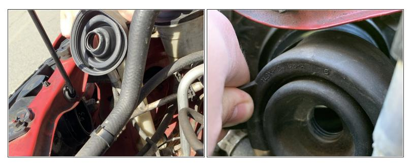
• Remove the rubber boot surrounding the housing. It will peel off when pulling the tabs to the side.
