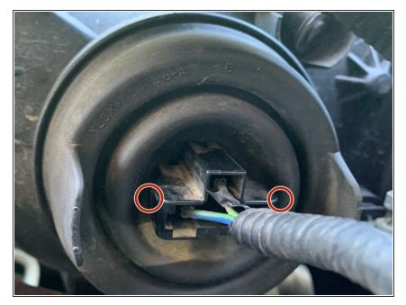
Push in on the sides of the bulb plug and pull directly out. It may take a bit of wiggling and effort to remove the plug.
