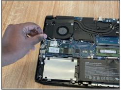
Remove the 2.6 mm screw that is holding down the SSD with a Phillips #0 screwdriver.
