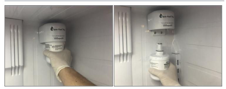
Twist the old filter towards "unlock" and pull down to remove the old filter.
