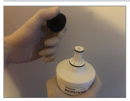
Get the new filter and remove the cap.
