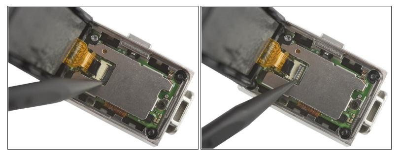
• Use the pointed end of a spudger to open the ZIF connector by pushing up the black flap.
