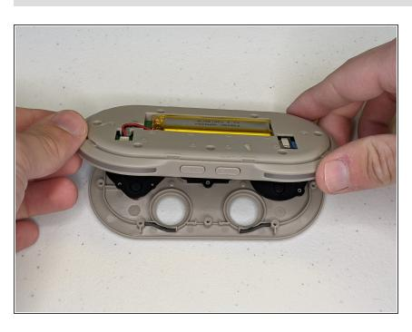
Lift the body of the controller up and away from the controller's face and buttons.
