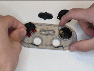
Lift away the black rubber pads that sit between the face buttons and body of the controller.
