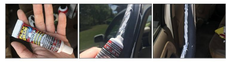
Once the cleaner has dried, take your silicone/ waterproof sealant and apply thick, evenly spread beads to the backside of the weatherstripping.
