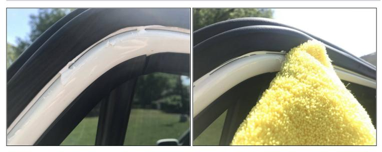
• Wipe away any excess adhesive with a clean microfiber towel that has been sprayed with brake cleaner.
