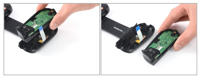
Remove the upper half of the left controller assembly.
