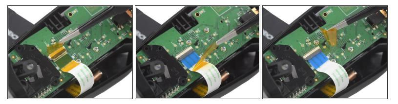
• Use a pair of tweezers to remove the yellow protective tape which is placed over the interconnect cable connector.
