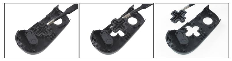
• Use a pair of blunt nose tweezers to remove the direction pad.
