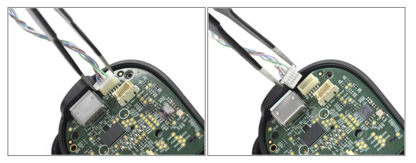
Use a pair of tweezers to disconnect the second phone connector cable from the mainboard.
