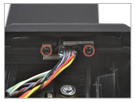
Use a Phillips screwdriver to remove the two 4.8 mm-long screws securing the phone connector.
