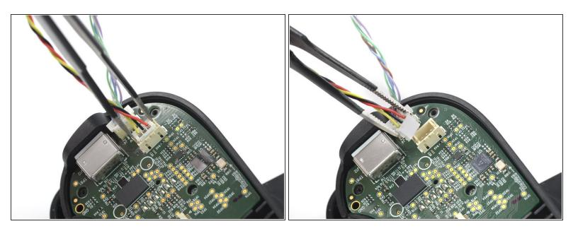
Use a pair of tweezers to disconnect the first phone connector cable from the mainboard.
