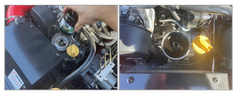
Remove the oil filter by turning it counterclockwise.
