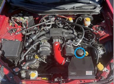
Open the hood of the car and locate the oil filter.
