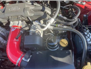
Screw the new oil filter in a clockwise rotation onto the same area where the old one was removed until it is tight.
