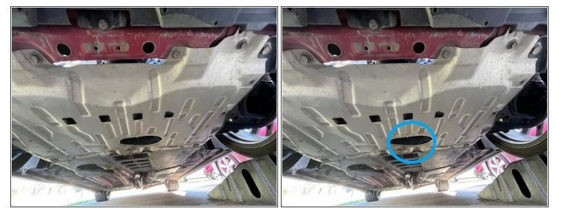
• Lie down under the front of the car and locate the oil drain plug in the opening on the skid plate.
