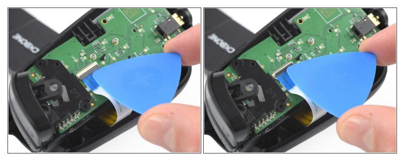
• Use the tip of an opening pick to open the gray flap of the ZIF connector by pushing it upwards.
