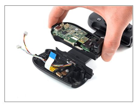
Separate the the upper case of the left controller handle.
