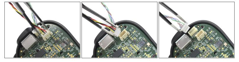
Use a pair of tweezers to disconnect the phone connector cables out from their sockets.
