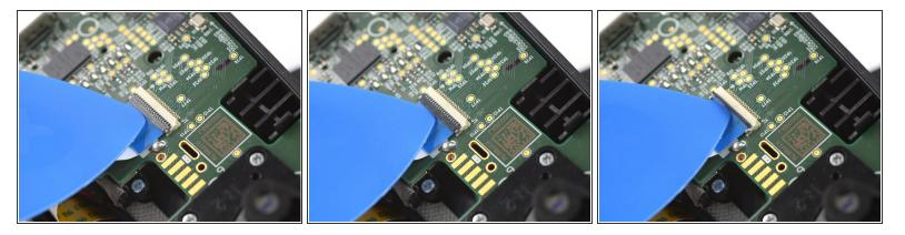
Use the tip of an opening pick to open the gray flap of the interconnect cable ZIF connector by pushing it upwards.
