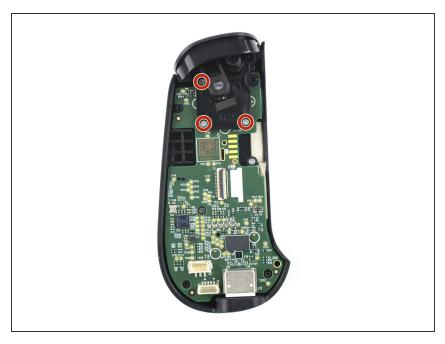
• Use a Phillips screwdriver to remove the three 5.9 mm-long screws.
