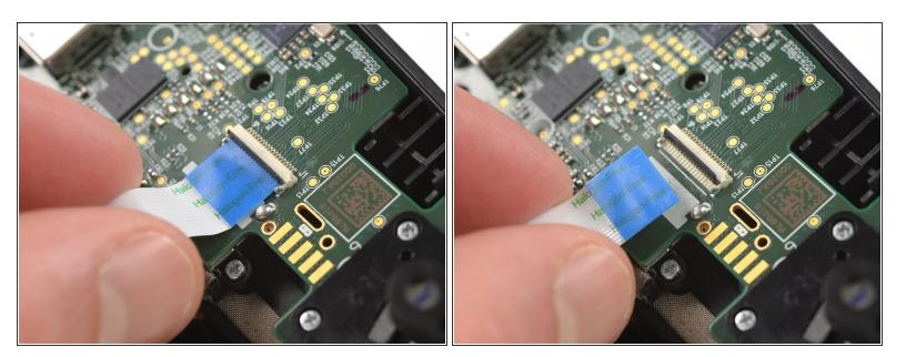
Disconnect the cable by pulling it straight out the ZIF connector.
