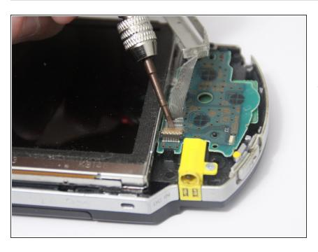
Disconnect the zero-insertion force (ZIF) connector by unlocking the locking tab with a plastic opening tool.
