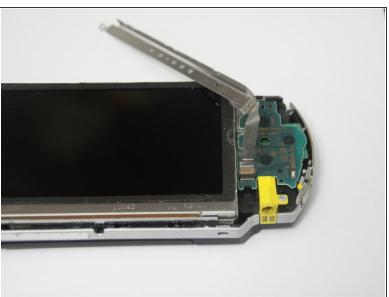
Using a plastic opening tool, lift the left side of the bottom circuit that includes the home, start, pause, and volume buttons.
