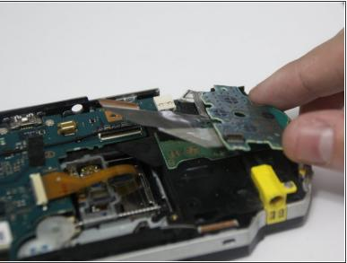
Use the plastic opening tool to unlock all of the ZIF connectors and disconnect all cables from the motherboard.
