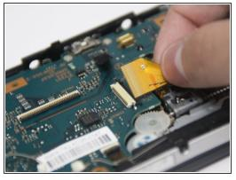
Using your fingers or a plastic opening tool, slide the UMD drive ribbon cable from the lock to release it.
