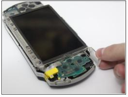
Remove the top left and right trigger buttons by simply pulling them out.
