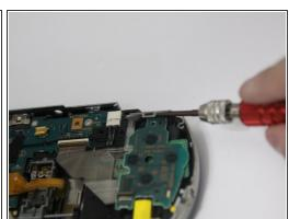
Using a plastic opening tool, remove the steel bracket under the right trigger.
