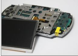
Use the plastic opening tool to unlock all the ribbon cables attached from the LCD screen to the motherboard.
