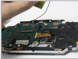
Above the charging input cable is the wireless antenna. Gently lift and place the wireless antenna
