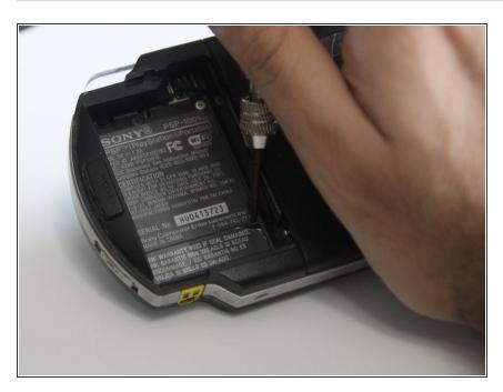
Using a flat tool, remove the warranty sticker. Removing this sticker will expose two screws.
