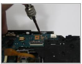
Using the Phillips #00 screwdriver, remove the single 4.4 mm screw located on the top right of the motherboard.
