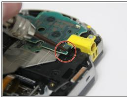
Using a plastic opening tool, unlock the small black clip that is located underneath the circuit board.
