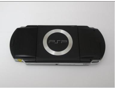
Remove any external cables from the device and place the device face down on a flat surface.
