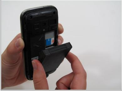
Remove the battery by pulling it away from the back of the phone.
