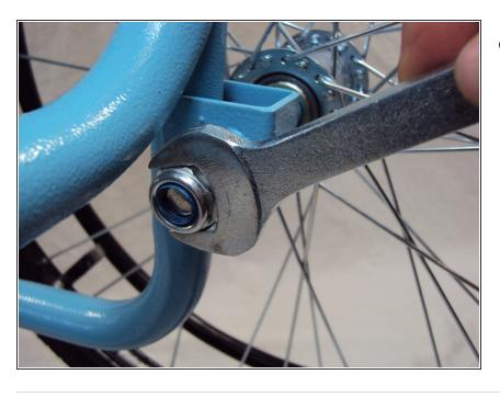
Tighten the nut facing the inside of the chair with a 19 mm wrench.
