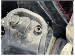
Using the Phillips #3 screwdriver, remove the two screws holding the bulbs.
