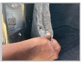
Peel away the trunk cover to reveal the two bolts holding the lights.
