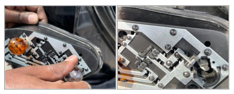
Take out the brake bulb by pushing it down and turning it counter-clockwise at the same time.
