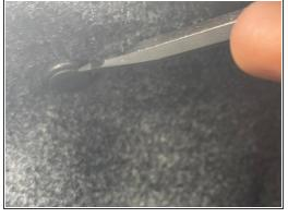
• Remove the two plastic pins holding the plastic trunk cover using the flathead screwdriver.
