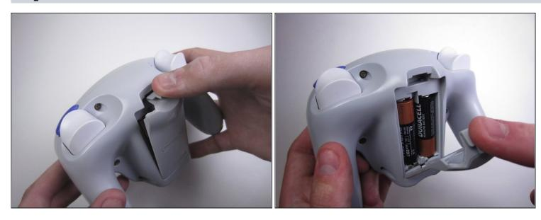
Pull down on the battery cover release lever and pull back to remove the cover.
