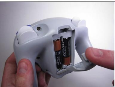
Pull down on the battery cover release lever and pull back to remove the cover.
