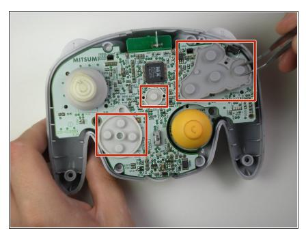
Using tweezers remove the three grey button pads from the motherboard.
