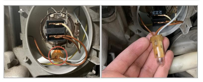
Pull the smaller lamp out. It has a grey wire attached to it.
