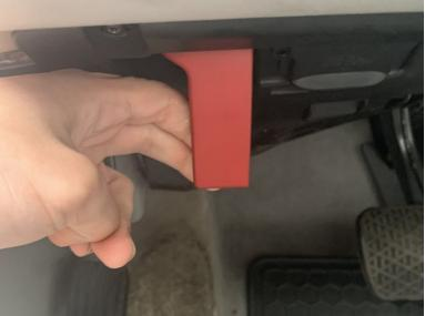
Open the car hood by pulling the red lever placed under the light switch.
