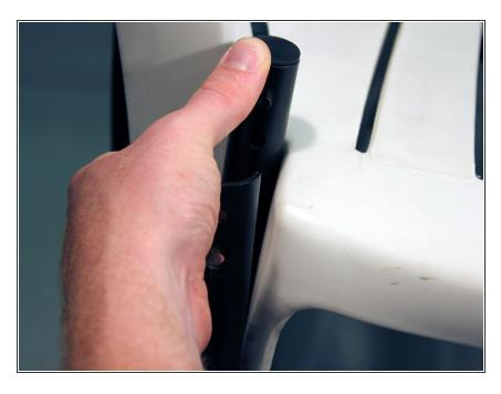
Remove the front frame and each of the castor wheels from the wheelchair.
