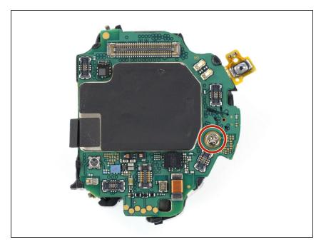
Use a Phillips screwdriver to remove the 4.4 mm-long screw holding the motherboard in place.
