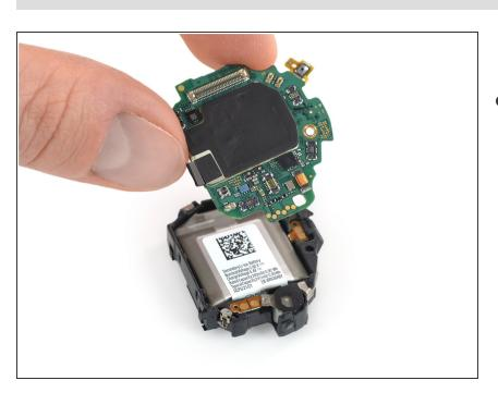
Slide the motherboard out from under the remaining plastic tabs to remove it.
