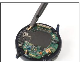
Use a spudger to disconnect the display assembly and the speaker.
